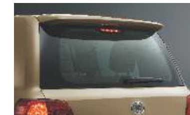
LED high-mount stop lamp brilliantly alerts drivers behind to impending stops.
