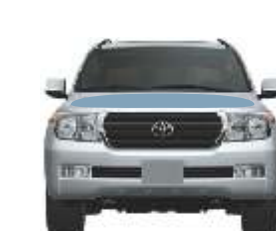
An impact-absorbing front hood/fender/cowl structure helps reduce impact on pedestrians.
