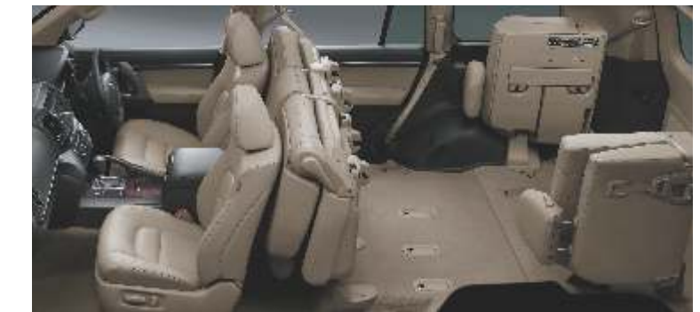
2 nd row seats tumble and 3 rd row seats fold laterally to maximise luggage space.
