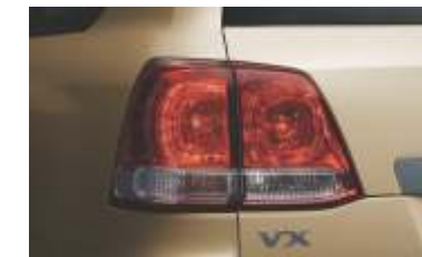
Rear combination lamps, LED-type tail and stop lamps are highly visible to the drivers behind.
