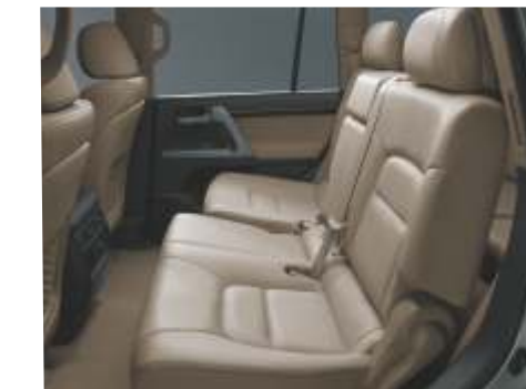
Seat-slide mechanism expands leg room for 2 nd and 3 rd row passengers.
