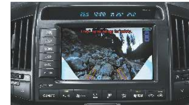
The back guide monitor with a Back Camera and linked display on the EMV Screen makes parking much easier and safe.
